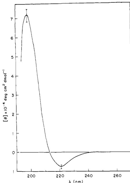
**Figure 1.** Circular dichroism spectrum of Cbz-Gly-L-Ser-(O-Bu')-L-Ser-Gly-O-stearyl ester in cyclohexane: concentration, 0.116 ~ 0.056 mg/mL; 1-mm cell; temperature, 23 °C.
