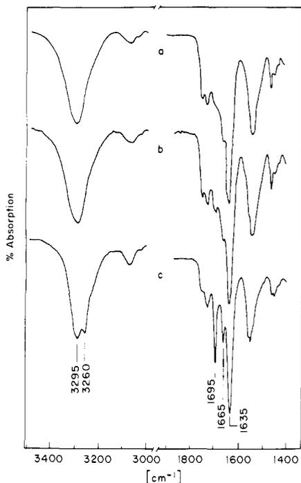
**Figure 3.** Infrared spectra of films of Cbz-Gly-L-Ser-(O-Bu')-L-Ser-Gly-O-stearyl ester cast from various concentrations in cyclohexane: (a) 3.54 mg/mL; (b) 0.290 mg/mL; (c) 0.060 mg/mL.
